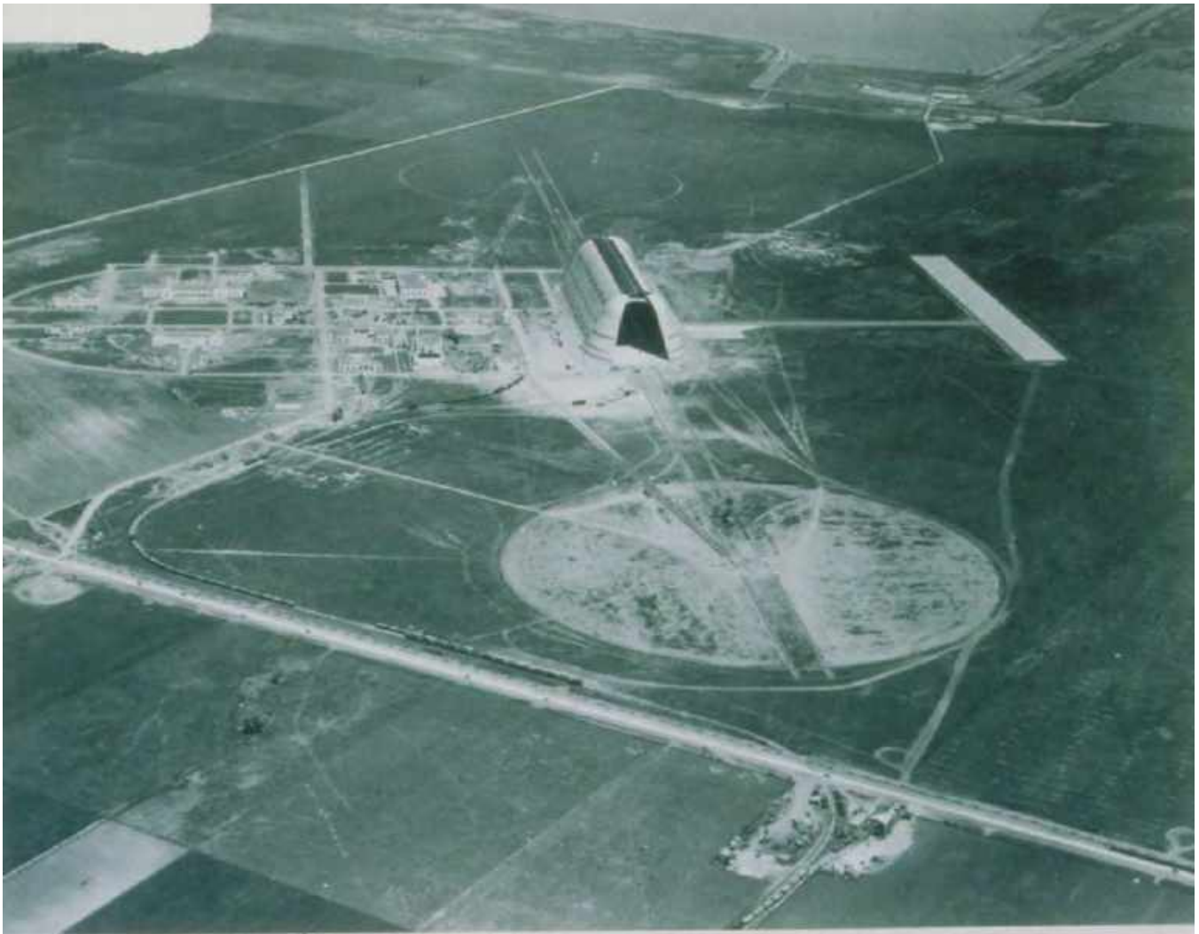
Early aerial photograph of NAS Sunnyvale showing Shenandoah Plaza at center left, Hangar 1 with the mooring circles for the USS Macon , and the original runway configuration for the Sparrowhawk planes at center right, c. 1933 (Source: Moffett Field Historical Society )
